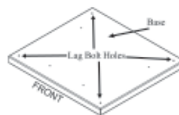
Figure 16C KSH Anchor Holes
